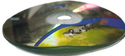
Figure 23. Example of a physically deformed optical disc
