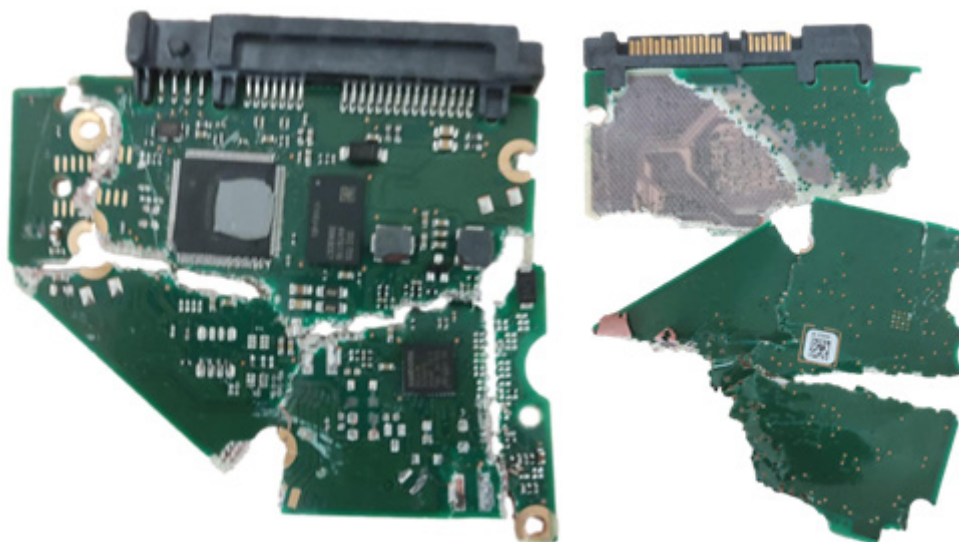
Figure 51. Intentional breakage of the printed circuit board
