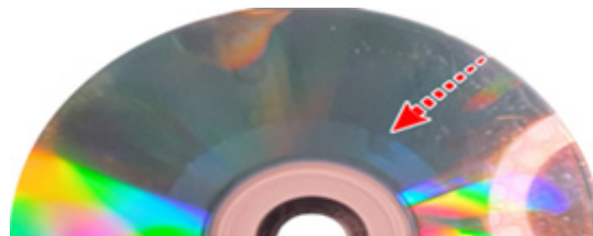
Figure 20. Error during data recording to optical disc
