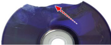
Figure 17. Fracture of the optic disc
