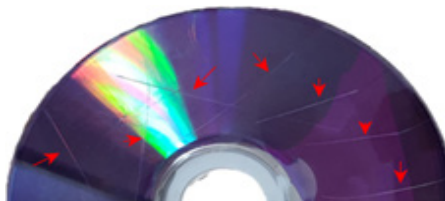
Figure 19. Having deep scratches on the optical disc
