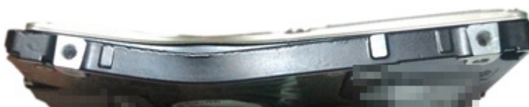
Figure 52. Physical damage to the disk (Recovery HDD, 2018)
