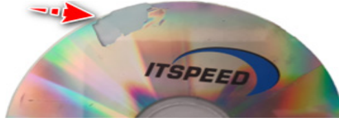
Figure 21. Wear of the reflective surface of the optical disc
