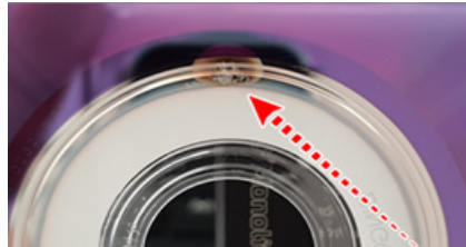
Figure 22. Optical laser burning of the optical disc
