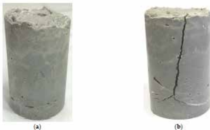
Figure 3. (a) Concrete cylinder representative for all samples and time periods except two Al containing cylinders (out of five) exposed for two years and (b) Concrete cylinder containing Al that cracked after two years of exposure.
