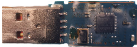
Figure 33. Oxidized USB flash drive
