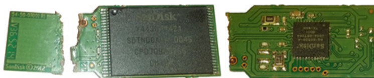
Figure 11. Breaking the USB PCB
