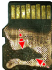
Figure 35. Excessive scraping of the memory card surface
