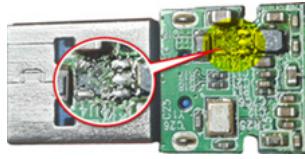
Figure 12. Fragmentation/loss of circuit element
