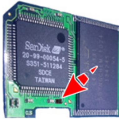
Figure 22. Deterioration of circuit elements on the memory card
