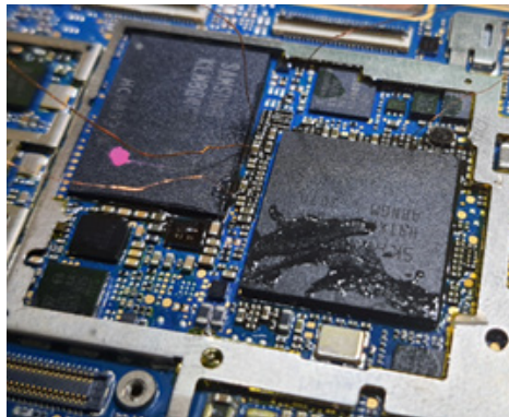
Figure 39. An example of ISP applied to a mobile device whose physical failure cannot be repaired
