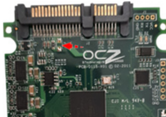
Figure 20. Example of fragment breaking from SSD
