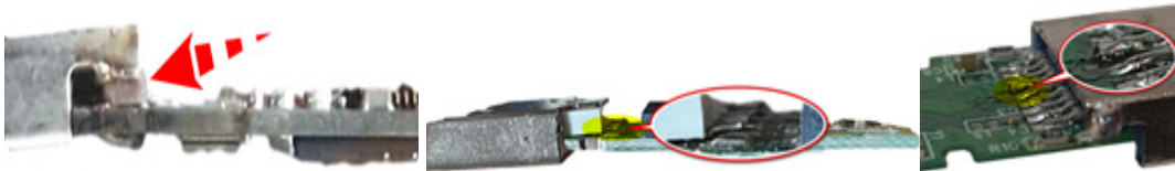
Figure 14. USB socket pins not touching
