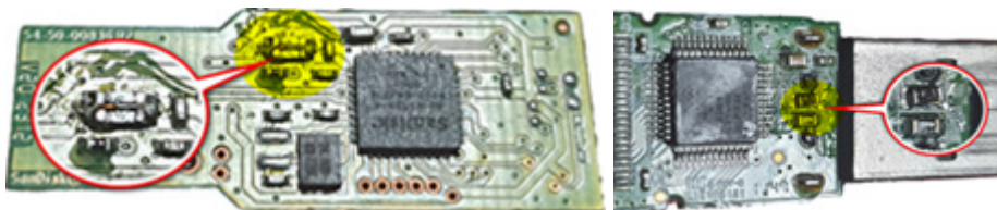
Figure 15. Bad fuse resistor
